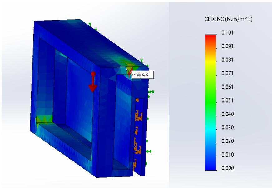
**Figure 21:** Strain Analysis of the Final Design
