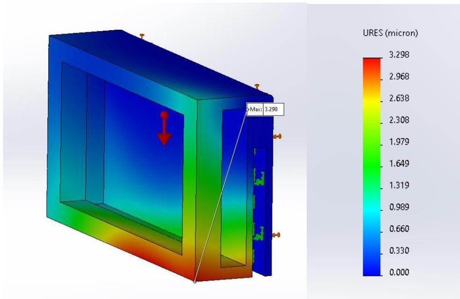
**Figure 23:** Displacement Analysis of the Final Design
