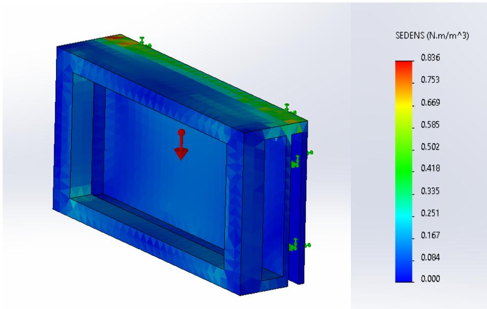
**Figure 20:** Strain Analysis of the Initial Design
