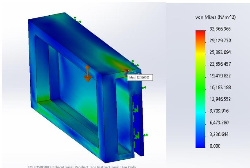
**Figure 19:** Stress Analysis of the Final Design
