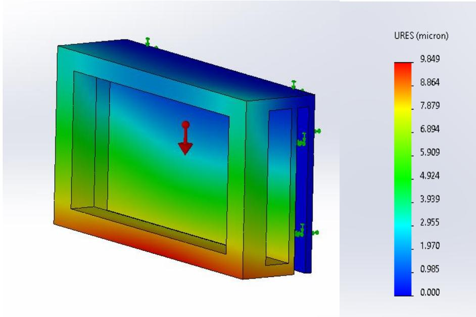
**Figure 22:** Displacement Analysis of the Initial Design
