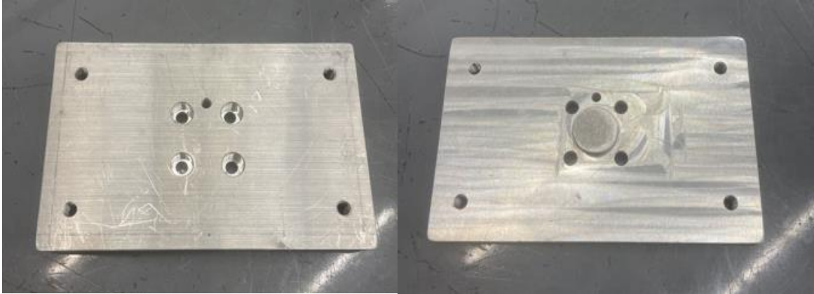
Figure 14: Finished Mounting Plate
